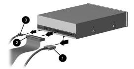
disconnecting the optical drive cables
